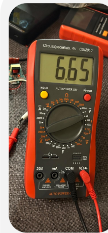
Typical peak continuous current draw. (Excluding propellor motors)
